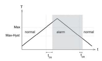
In the normal state the integrated LED is on, in the alarm state it is off, and this corresponds to its status when there is no auxiliary voltage.
